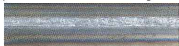
Fillet weld(mild steel, 1.0mmt) [Welding current:80A, Welding voltage:18V] [Wire dia.:1.2mm, Shielded gas:CO 2 ]
