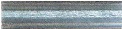
Fillet weld (mild steel, 1.0mmt) { Welding current : 80A, Welding voltage : 18V } { Wire dia. : 1.2mm, Shielded gas : CO 2 }
